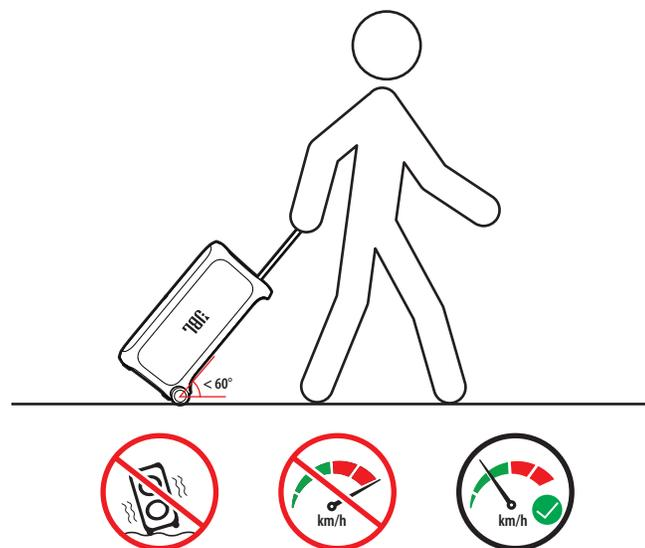
To avoid tip-over, do not drag the speaker on uneven surfaces or slopes where stability is doubtful. Stop or slow down when you feel any wiggle in the wheels.
